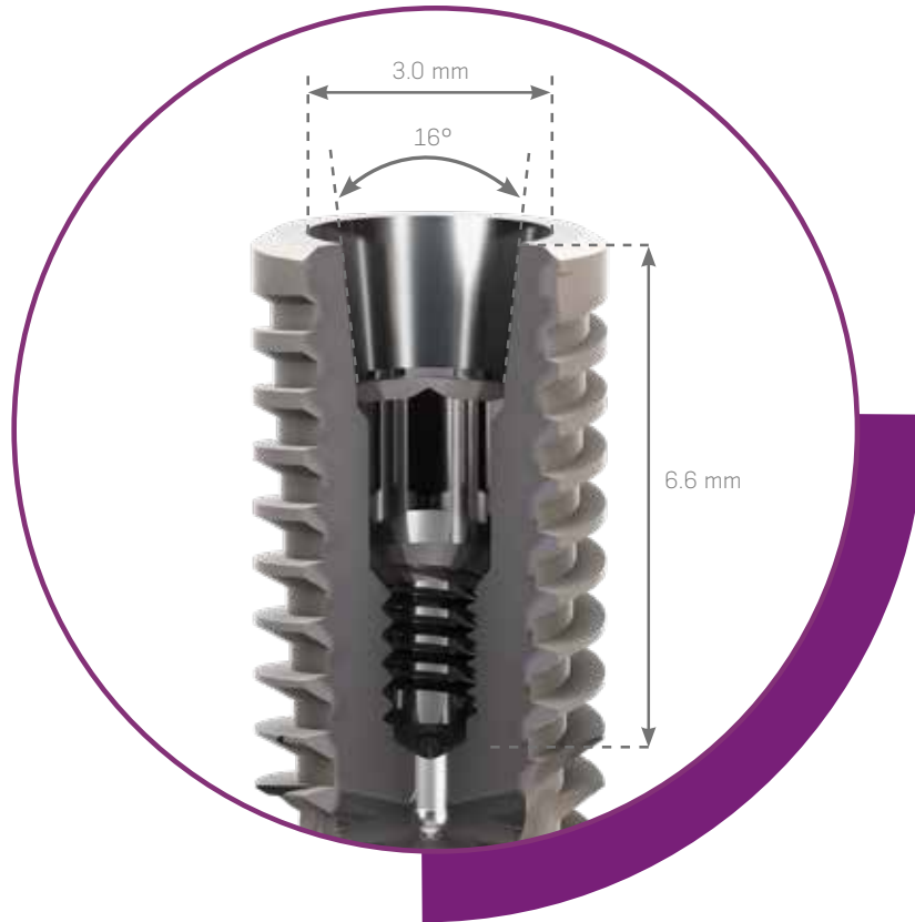
FIGURE 1. The Neodent® Grand Morse™ Implant has a deep tapered connection on the inside of the implant, which is designed to increase the contact area between the implant and the abutment. In addition, this connection has a larger diameter, resulting in a simpler, more efficient clinical procedure.
