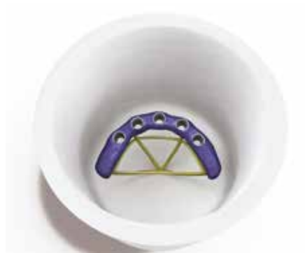
11) Castable ring with waxed framework.
