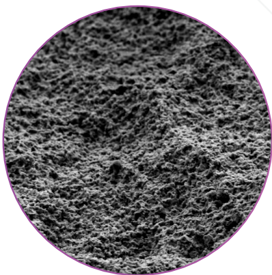
Representative image of the implant surface - Scanning Electron Microscope (SEM) magnification of 5000x.
