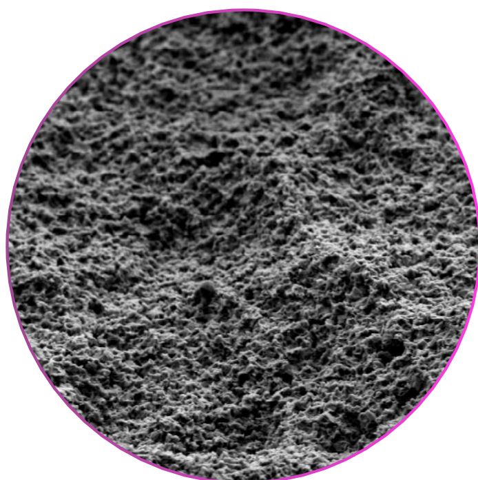
Representative image of the implant surface - Scanning Electron Microscope (SEM), magnified 5000x.
