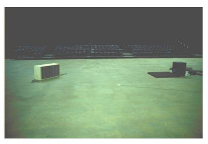
analyzer. We also drew a concentric 30' radius semicircle with similar angular steps for the loudspeaker, so that we could measure the polar scattering for different angles of incidence. Needless to say, this was a physical and tiring process, because we also had to move ourselves out of the area of detection, so we were not in the measurement. These measurements also had to be done very late at night when the arena was not being used. Soon, the owner lost patience and we had to find another
