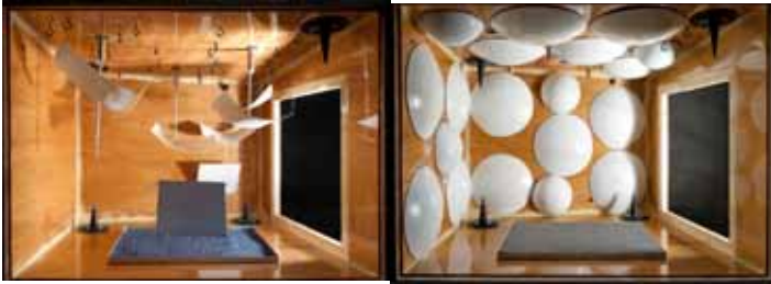
Figure 3.4. Top: Traditional suspended ceiling diffusers, which reduce mean free path and room volume in unpredictable ways. Bottom: Suggested boundary mounted diffusers allow accurate calculation of the room surface area and volume. Lautenbach & Vercammen, Proc. 20th ICA 2010.
