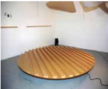
Figure 1.2 Scattering Coefficient ISO 17497-1: How much of the incident sound is scattered away from the specular zone (Can be measured in scale and calculated).
