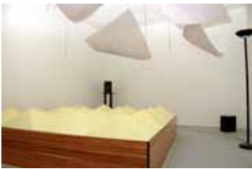
Figure 1.1 Absorption Coefficient ISO 354: How much of the incident sound is absorbed (Must be measured full scale).
