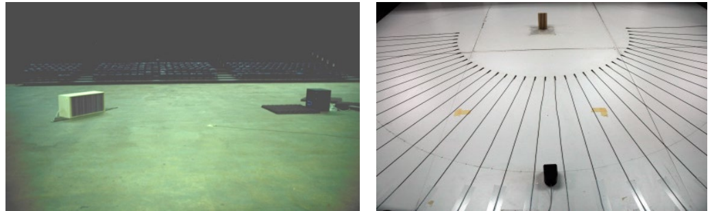
Figure 8. Left: Full scale measurements in a sports arena; Right: First scale model goniometer
