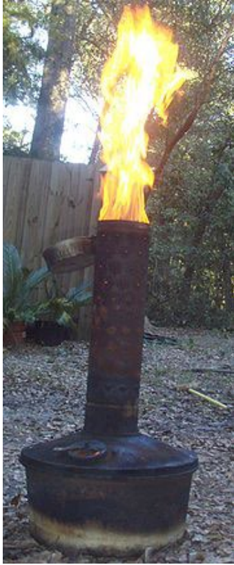
Oil-burning smudge pot, used to protect temperature-sensitive citrus groves from freezing temperatures.
