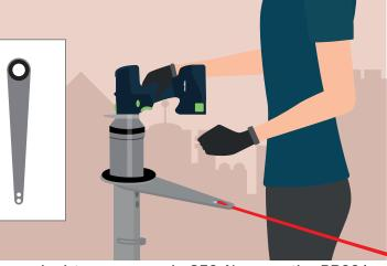
If the required torque exceeds 350 Nm, use the BR001 reaction arm.
