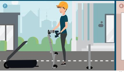
Connect the actuator to the foot held reaction arm (BA012)
