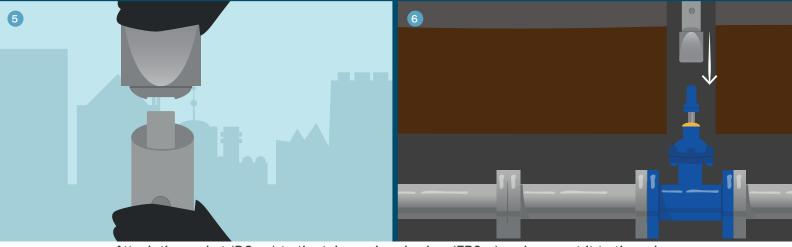
Attach the socket (DCxxx) to the telescopic valve key (EB0xx) and connect it to the valve. The top of the valve key must be at thighs level.
