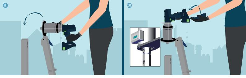
Plug the actuator to the valve key, adjust the height of the BA012 to be comfortable.
