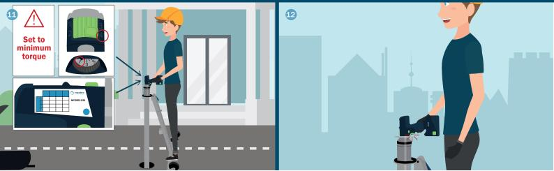
Set torque to minimum, select rotation direction (D1=Clockwise/D2=Counter-clockwise) and start the operation. Increase torque and/or speed if necessary.
