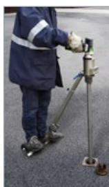
Example of use with a buried / underground valve.
