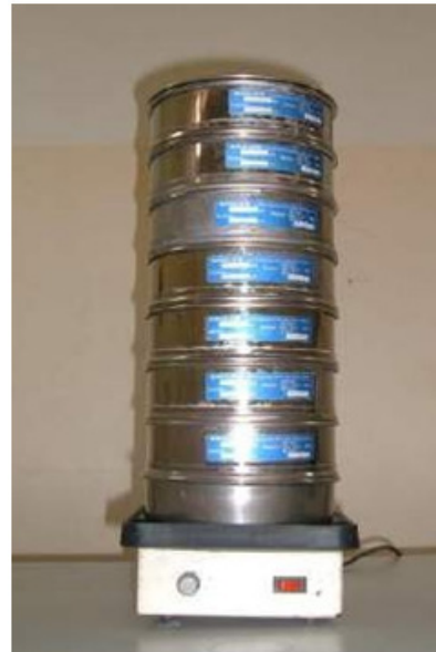
Figure 1: Laboratory sieve on vibrator
