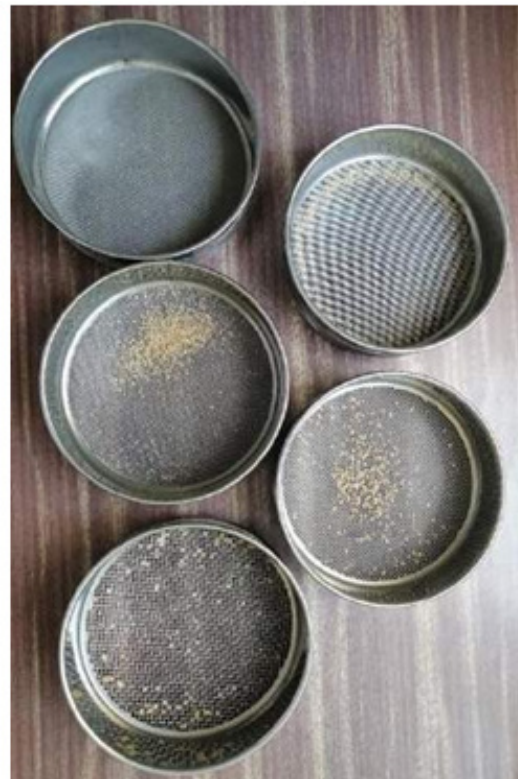
Figure 2: Top view of sieves after vibrating.
