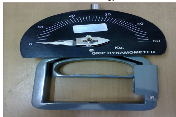
Figure 1 showing hand grip dynamometer to measure MVC
