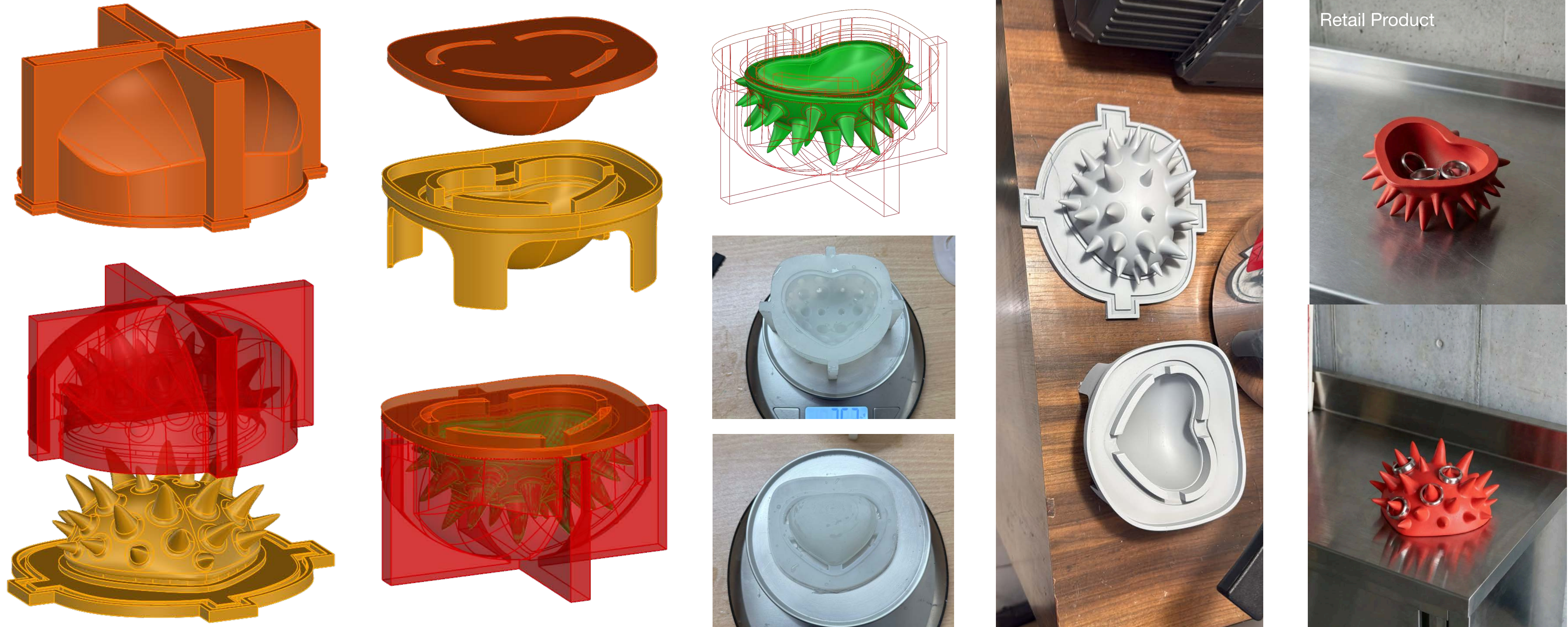
03 Part SLA reverse moulds for silicone mould: This mould was used to produce multiple silicone moulds, helping speed up production by overcoming resin curing time limits. The reusable master mould allowed several silicone moulds to be made, which then enabled multiple resin parts to be cast simultaneously.
