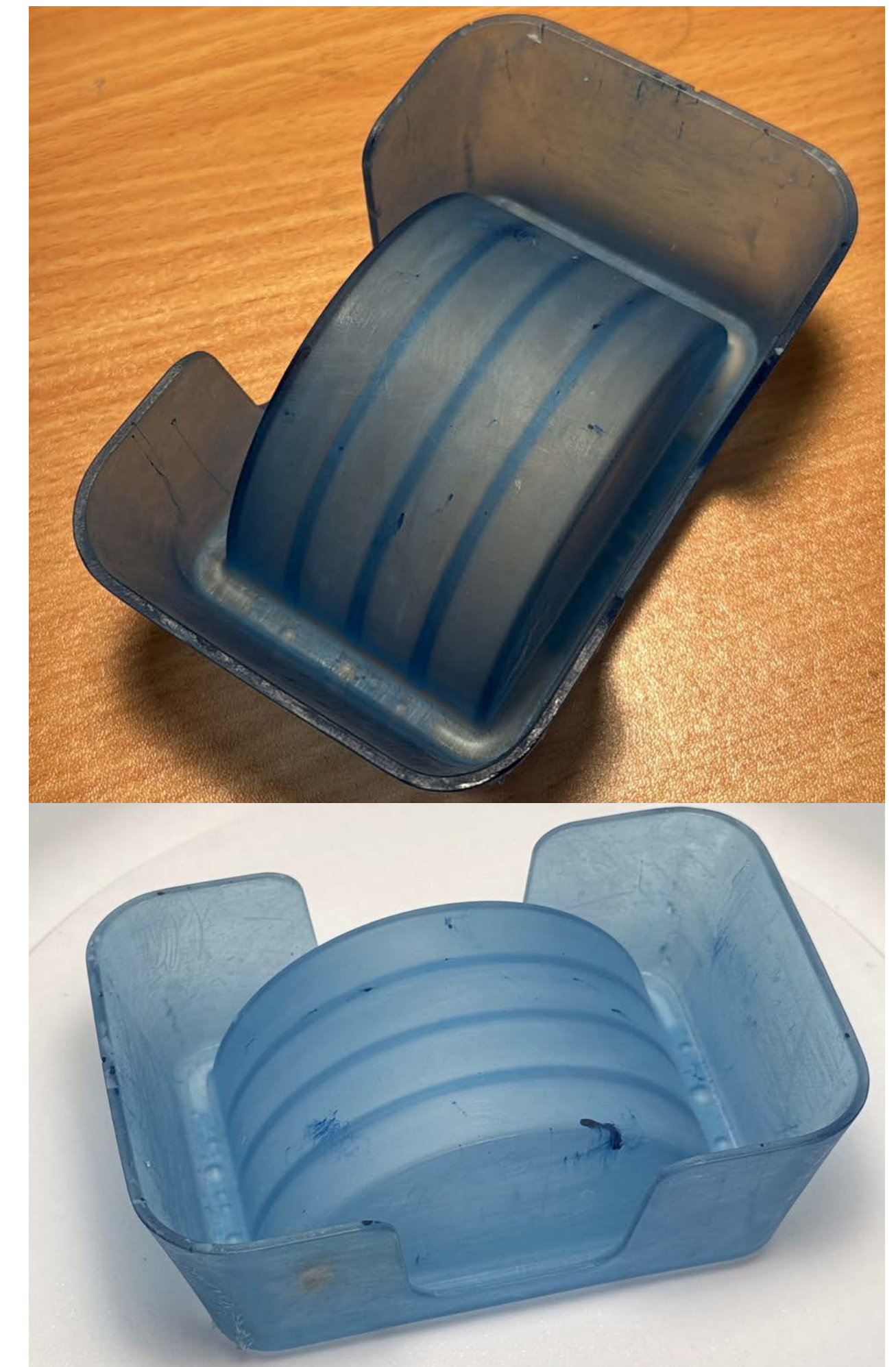
Casted Part [80mmX50mmX28mm]
