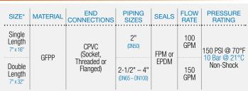
\* PVC and CPVC socket ends available to ISO 727-1 and threaded ends to BS21. PP socket fusion ends per ASTM F2389 and threaded ends per BS21. Flanged ends available in DIN/EN PN10.
