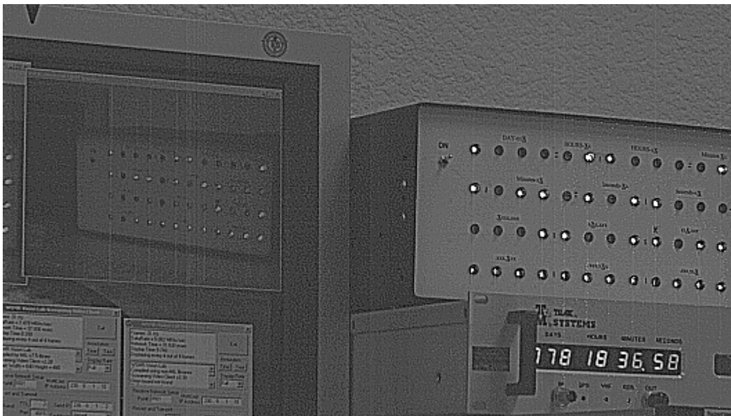
Figure 5: High speed image frame shows ~190 millisecond round trip cross country latency.
