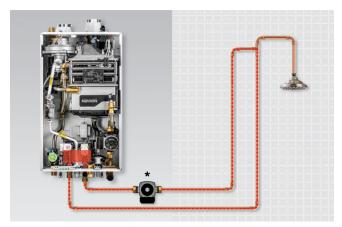
\*A dedicated recirculation line and external recirc pump are necessary and not included. See installation manual for details.
