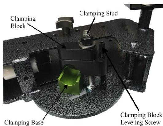
1. Find the appropriate clamping base that matches the tube diameter and place the bottom pin into the short slot on the frame of the cutting attachment.
