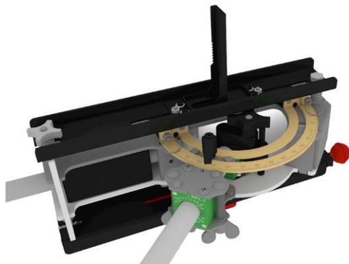
The miter attachment has two tracks - one above and one below the cutting area. The upper track has a sliding car fit with the reciprocating saws pivot shoe. *(If not installed, attach the pivot shoe onto the sliding car with the 4 fasteners & washers making sure the saw, when attached, cuts from left to right.)*
