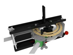
The miter attachment has two tracks - one above and one below the cutting area. The upper track has a sliding car fit with the reciprocating saws pivot shoe. (If not installed, attach the pivot shoe onto the sliding car with the 4 fasteners & washers making sure the saw, when attached, cuts from left to right.)
