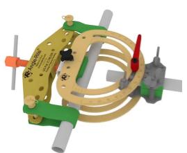
Attach both clamp halves mounted in the guide plates (J) over the tube and pivot the bolts into the slots on the other clamp half guide plate. Make sure the brass washer (M) is between the wingnut and the steel plate. The cupped washer (N) should be between the plate and the end of the spring. Tighten the two wingnuts evenly so that the guide plates holding the clamp halves are parallel to each other.
