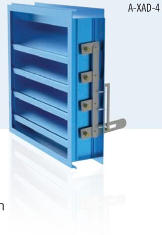
**The A-SL series** of formed steel louvers provide all the features and benefits of the fixed blade versions of the SL series louvers, but include the added feature of adjustable blades. The adjustable (operable) louvers allow for the weather protection of a louver when open and can provide positive shut off when no airflow is required.
