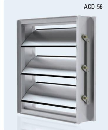
**The SCD series** of control dampers have been designed and tested to provide a reliable and cost effective control damper. Fabricated of roll-formed galvanized steel frames and blades, the SCD series features concealed linkage and is available in either parallel or opposed blade operation.
