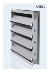
**The HDB series** of heavy duty backdraft dampers are designed for higher pressure, velocity or temperature environments. Dampers are fabricated of heavy gauge galvanized steel standard; these dampers are capable of operating up to 250°F and up to 3,000 fpm (HBD-H).
