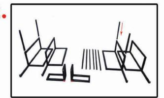
Place two (2) insert pieces with center indicators facing up into the slots of two corners as shown.
