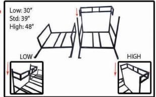
Lay sections flat. Insert final (4) pieces and install top assembly. For low position, turn top assembly over.
