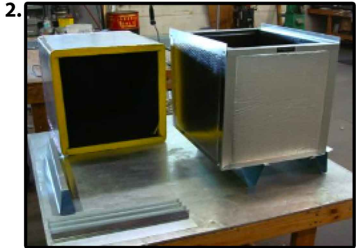
Assemble Side-Return Box, and tape seams. Note: Fiberglass Return Air Handler Stand and Qty: 2 V-Legs sold separately.
