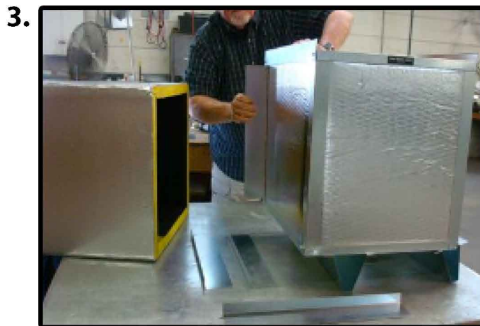
Cut hole in Return Air Stand. Slide the Start Collar under metal frame
