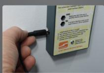
**STEP 6** Plug the current sensor wire into the jack on the Remote Indicator Panel.
