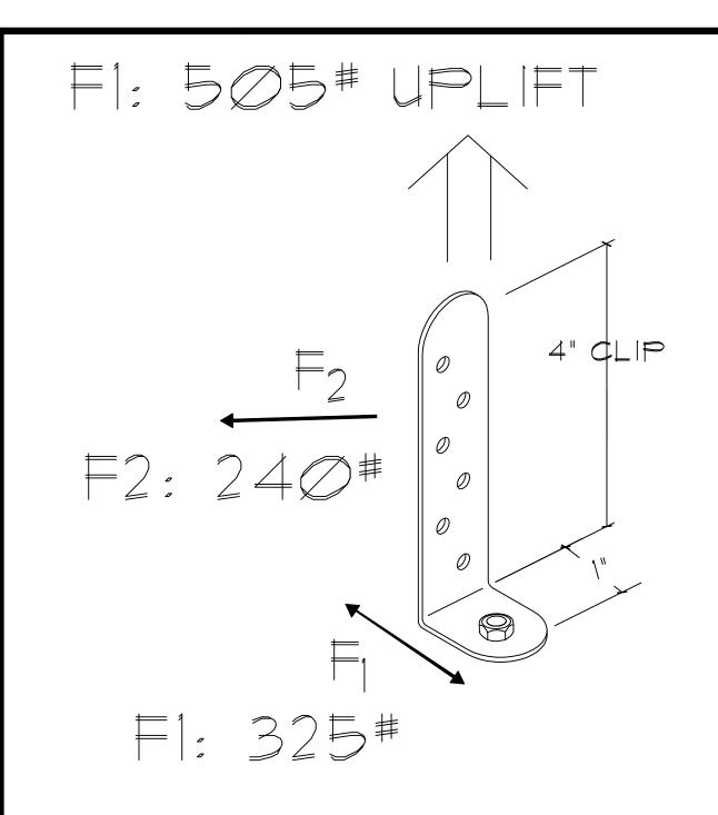
USE MIN. OF 4-  $\#10\times3/4$ " SCREWS FOR 4" CLIP TO CONDENSER USE MIN. OF 4-  $\#10\times3/4$ " SCREWS FOR 6" CLIP TO CONDENSER USE 1/4"  $\times1$  3/4" TAPCON STAINLESS STEEL TO CONCRETE PAD
