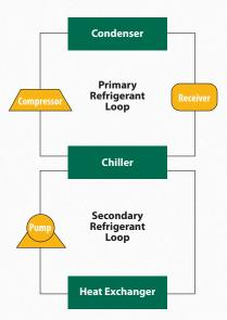
The primary loop consists of a compressor and air-cooled condenser. The liquid refrigerant flows from the condenser to a heat exchanger, which is the primary system evaporator, and is controlled by an expansion device. The refrigerant leaves the heat exchanger as superheated vapor and is circulated back to the compressor.
