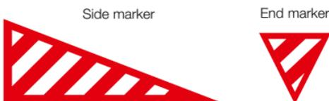
Both required when load or equipment (eg crane jib) overhangs front or rear by more than two metres
