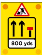
Signs used on the back of slow-moving or stationary vehicles warning of a lane closed ahead by a works vehicle. There are no cones on the road.
