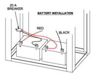
13. Decide if the breaker should be located on the left or right side of the tower. Un-screw the outer locking nut, insert the breaker button through the large hole on the side panel at the rear mid-section of the tower, on the side selected for the breaker, and re-install locking nut to secure.
