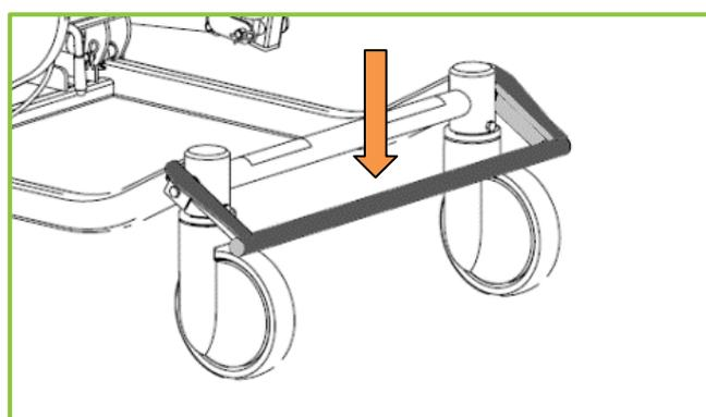
Figure 33 – Brake locked
