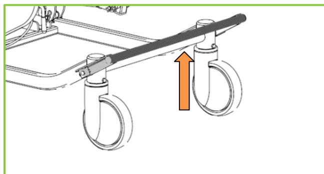
Figure 34 – Brake unlocked
