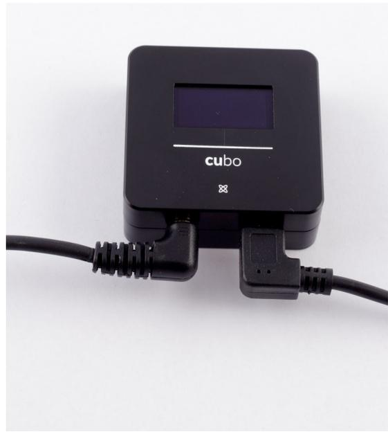
*Headrest Sensor Connector    Link Connector*
