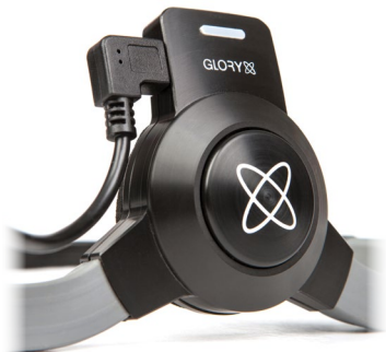
Connecting the Data cable to the GyroSet Link
