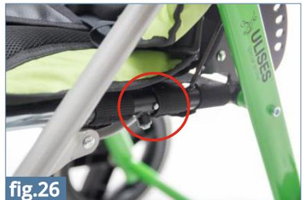
Maximum depth setting of the seat is indicated by the retaining pins coming into holes located at the both side of the seat frame. To decrease the seat depth, after reaching its maximum position, push the retaining pins inside the frame.
