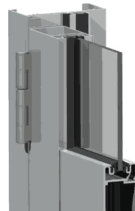
**Figure 3.9: Section through door base, hinged side**
