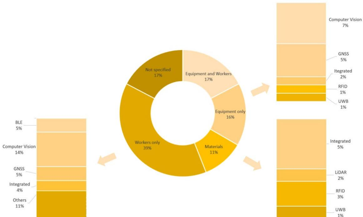
**Figure 5.2: Tracked resources in the review literature: the composition with tracking technology breakdown (2000 to 2021)**
