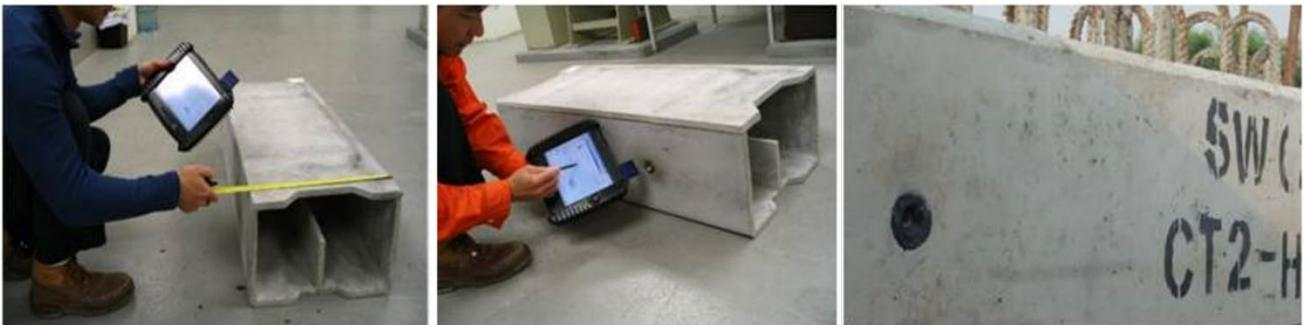
**Figure A9: Precast concrete identification and tracking** <sup>221</sup>
