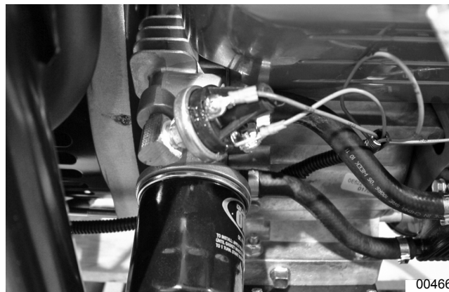
Figure 5-22. Low Oil Pressure Switch
