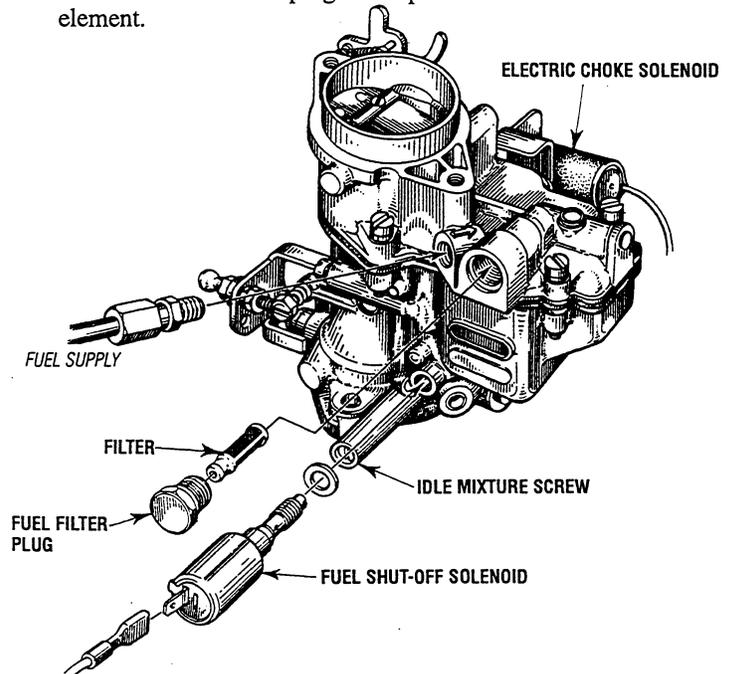
20. Make certain all the carburetor screws are properly tightened. Fasten the assembled carburetor on the intake manifold using new gaskets (use sealant). Replace the two nuts and washers and tighten the carburetor to the manifold.
