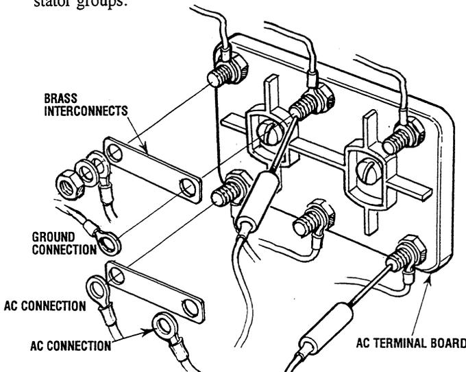
**TESTING MAIN STATOR WINDINGS**
