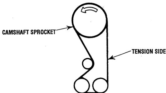
7. Loosen the temporarily tightened tensioner nut on the water pump side 1 or 2 turns, and tension the belt making use of the spring force.
