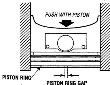
Check the piston ring for damage, wear, seizure and bends replacing the rings if anything unusual is noted. Always replace the piston rings when installing a new piston.
