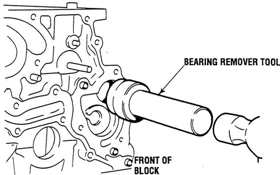
5. Use the same tool and drive the counterbalance shaft rear bearing from the cylinder block.
