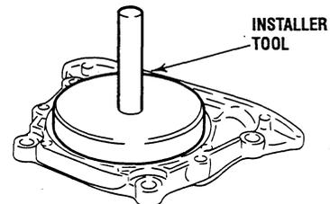
3. Install the oil seal case into the cylinder block through the gasket. (If there is no gasket, coat with sealant.) The entire circumference of the oil seal lip should be coated with clean engine oil.
