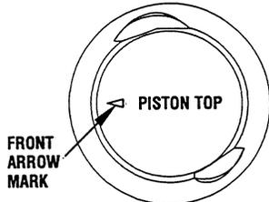
Securely pressing the piston ring with the ring band, insert the piston and connecting rod assembly into the cylinder. Keep in mind that the piston ring may be damaged if hit too strongly.
