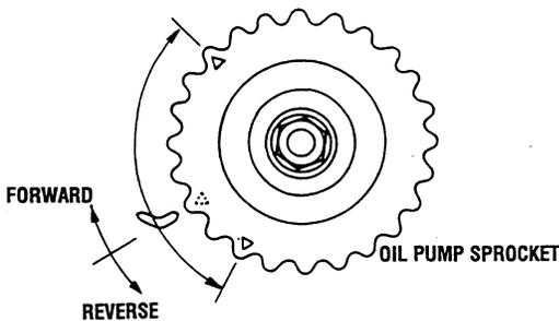
4. If the movable range of the teeth on the oil pump sprocket exceeds the specified range, correct as follows:
