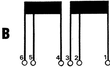
**NOTE:** The studs on the AC terminal board are identified by the six red wire that attach to them. These wires are numbered 1 thru 6. There are no numbers on the terminal block.
