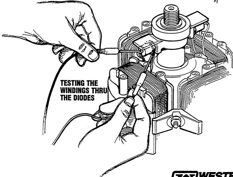
TESTING THE WINDINGS THRU THE DIODES
