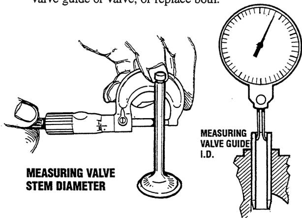
MEASURING VALVE STEM DIAMETER
