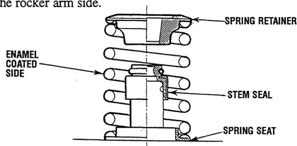
Use the valve spring compressor to compress the valve springs. With the valve spring compressed, remove the retainer locks.
