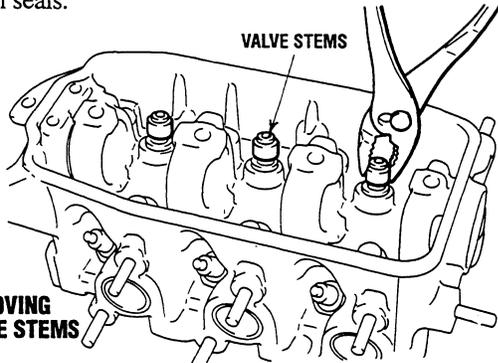
**REMOVING VALVE STEMS**
