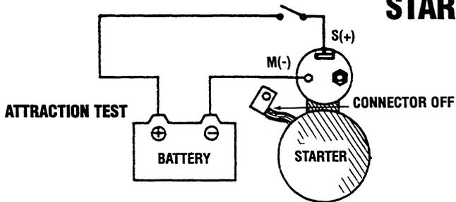
3. *Holding test.* With a battery connected to the solenoid terminal S (+) and to the starter body, manually pull out the pinion fully. The pinion must remain at that position even when released from holding with your hand.
