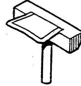
**CRANKSHAFT REAR OIL SEAL INSTALLER**
