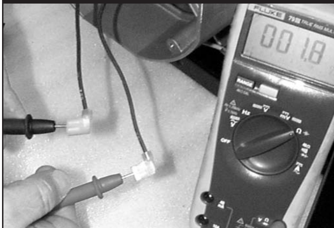
Figure 3.24 — Checking DPE Resistance
