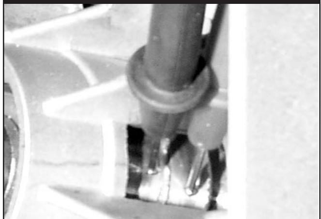
Figure 3.20 — Checking Rotor Resistance
