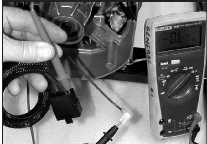
Figure 3.25 — Testing For Short Between Windings
