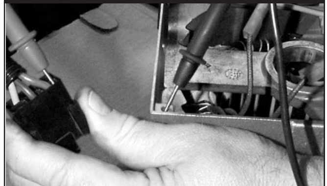
Figure 3.55 — Testing For Short To Ground
