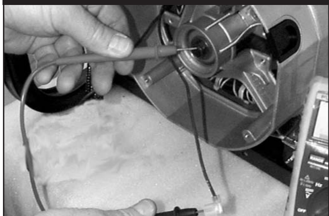
Figure 3.26 — Checking DPE “Short To Ground”
