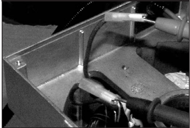
Figure 3.51 — Checking Excitation Resistance
