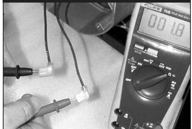
Figure 3.41 — Checking DPE Resistance
