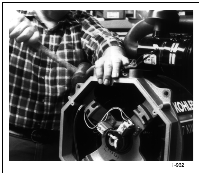
Figure 8-10. Removing the End Bracket
