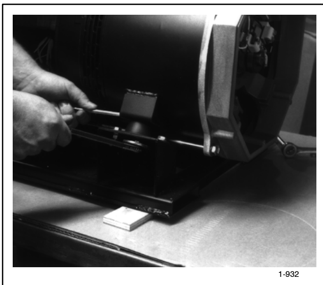
Figure 8-7. Removing the Vibromounts
