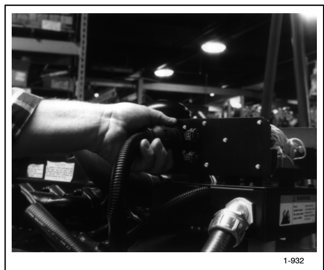
Figure 8-2. Disconnecting the 22-Pin Connector
