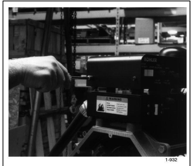
Figure 8-1. Removing the Controller Cover
