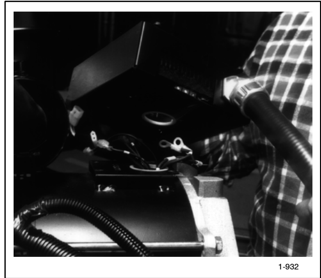
Figure 8-4. Removing the Junction Box
