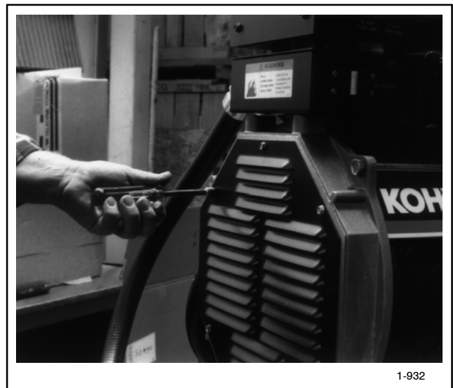
Figure 8-5. End Bracket Removal
