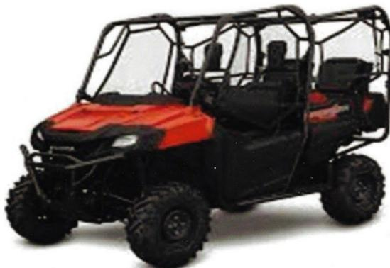
The Pioneer has A 675cc liquid cool engine, automatic transmission,
