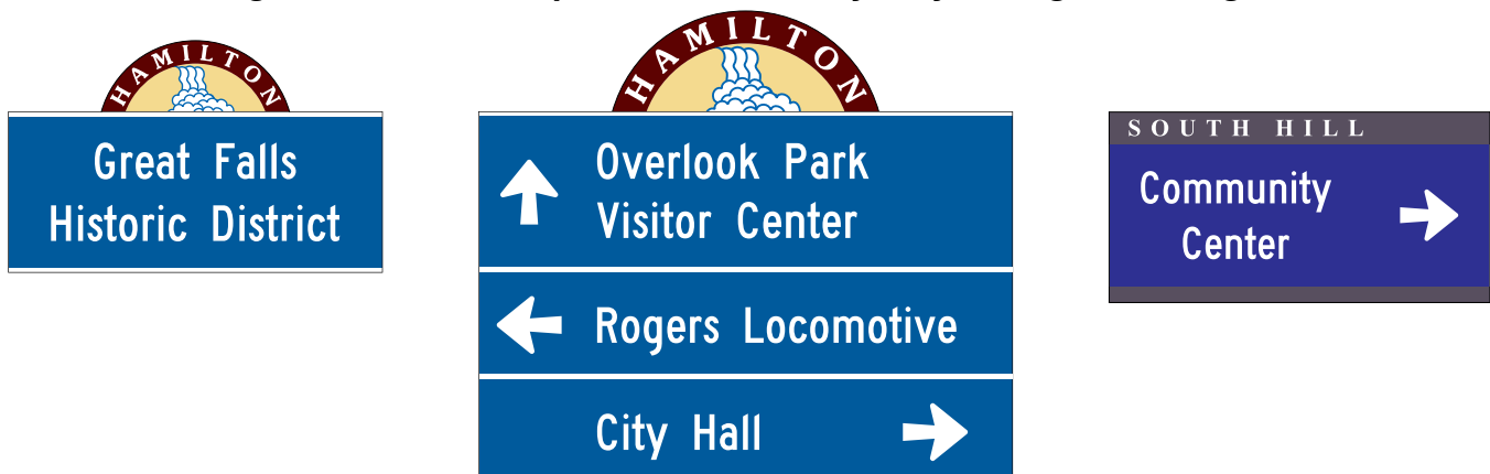
Figure 2D-30. Examples of Community Wayfinding Guide Signs
