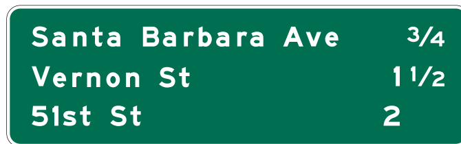
Figure 2E-10. Example of an Interchange Sequence Sign
