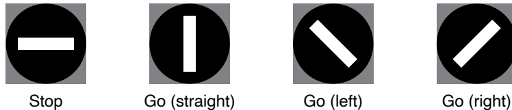
Figure 8D-3. Light Rail Transit Signal Indications
