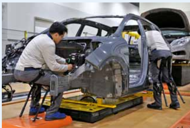
Exoskeletons at work. Hyundai’s Chairless Exoskeleton (H-CEX) is among the first to be used in car manufacturing, reducing strain on the workers (photo provided by Hyundai Motor Company).
