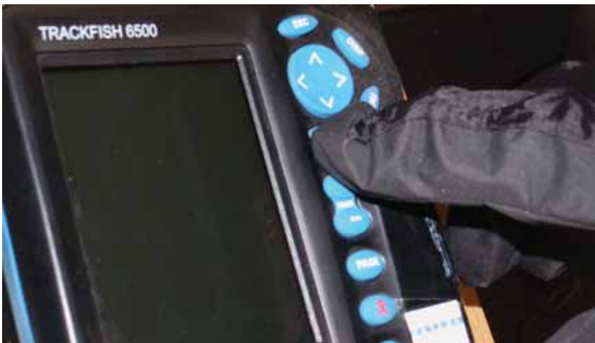
Figure F-2b An example of the difficulty of operating COTS marine displays when using gloves. Image copyright: Human Sciences & Engineering Ltd
