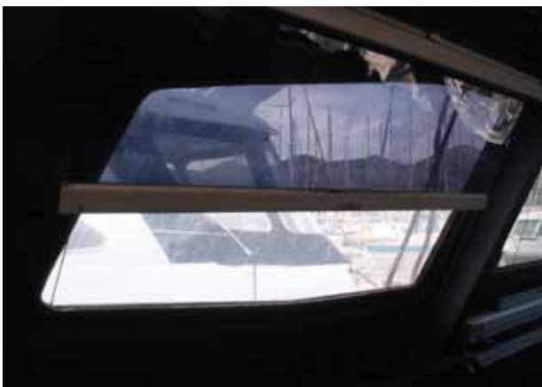
Figure B-4 Example of an antiglare shade being used on the inside of a HSC window
