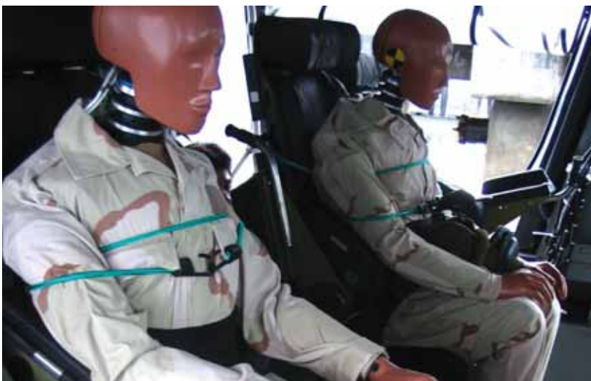
Figure J-6 Example of Anthropometric Test Dummies being using for the testing of the Stidd/Taylor V5 suspension seats fitted to the USN MkV SOC. Image copyright: US Navy
