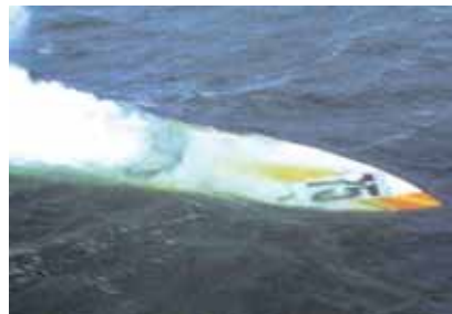
Figure E-2 Example of a submerging HSC demonstrating the need to include escape and evacuation design features as well as ensuring the HSC has the appropriate structural strength.
