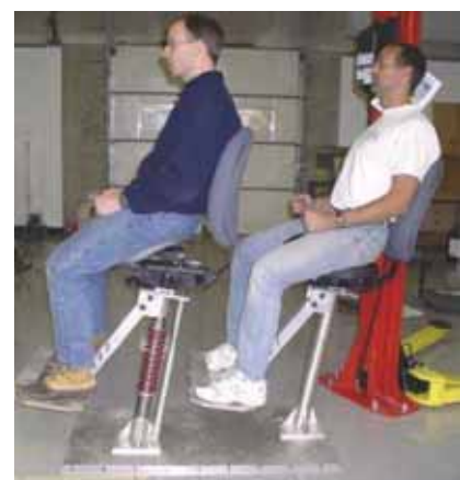
Figure K-7 Physical Mock-up for Evaluation of Proposed Postures.
