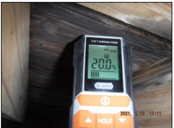
Moisture damage/elevated moisture - bathroom area
