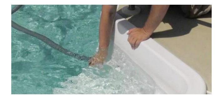
**NOTE:** Bubbles will come up from the vacuum head on the floor of the pool. Once the bubbles stop, all the air is out of the hose.
