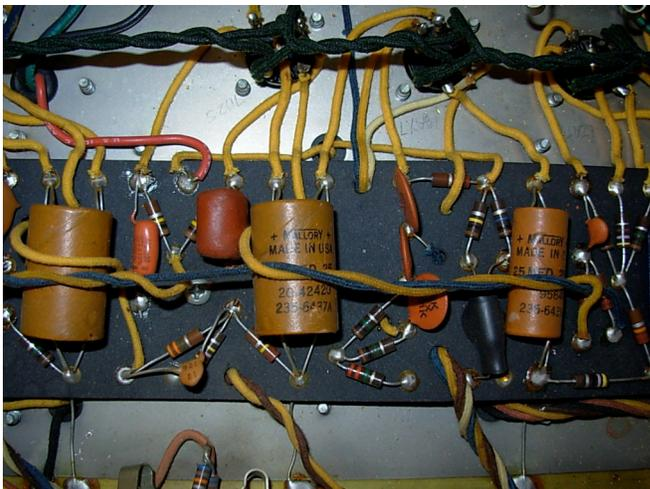
**Look at the dates on the capacitors. They weren't even made until the 37<sup>th</sup> week of 1964. With FENDER inventory stocking and normal delays this could not be a 1964 board.**
