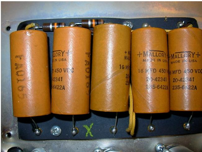
**Look at the filter cap board. Caps made the 22<sup>nd</sup> week of 1964..... Remember assembly delay and then look at the Assemblers number and date. 0165 – this board was assembled in January of 1965.**
