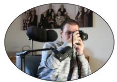
The arm support does not take over any function, the user moves themselves. The Armon simply supports the arm, however unlike a normal armrest, the Armon will dynamically 'follow' the position of the arm through space, providing full support in any position.
