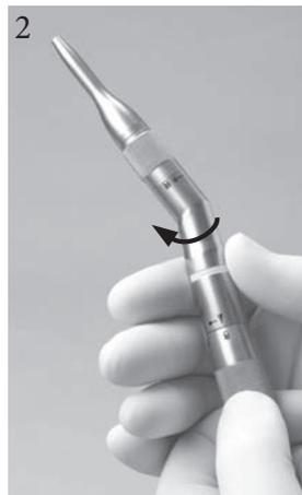
3. With “Tool Lock” in the “
