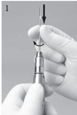
2. Slide footed attachment over dissecting tool onto motor aligning triangular arrows on attachment and motor case.
