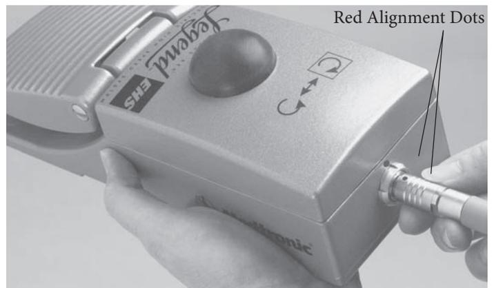
The Legend EHS Foot Control Cable Boot and the console’s foot control receptacle are both color-coded gold. Connect either end of the Legend EHS Foot Control Cable, by aligning the red dots, to the Legend EHS Foot Control Unit.
