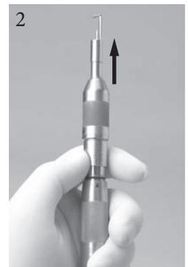
3. Pull dissecting tool out of motor collet and discard tool.
