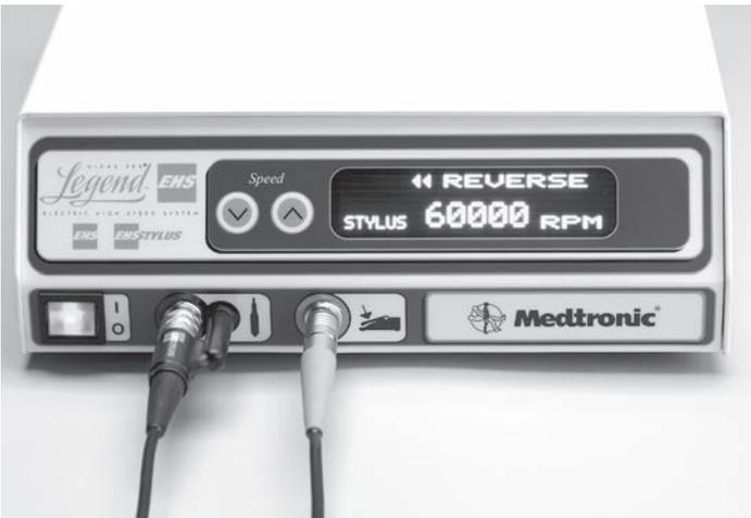
To return to forward rotation of the motor, stop the motor and step on the reverse button at the foot control. The console's digital display will indicate that forward rotation has been selected.
