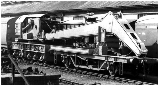
V Steam Driven Crane
