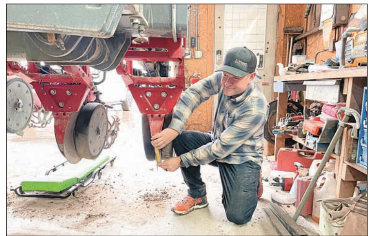
Michael Goodson inspects a 12-row bean planter's opening disc, which opens a uniform trench in which to plant seed, Feb. 24 near Parma, Idaho. Brad Carlson/Capital Press
