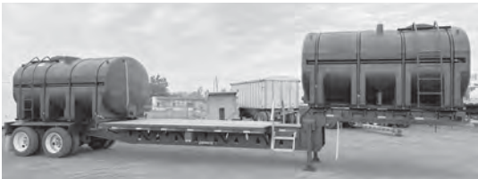
2024 DEMCO LIQUID TENDER , 42’ LONG, 3250-GAL FRONT AND REAR TANKS, AIR AND ELECTRICAL TO BOTH TANKS, 24” PIN SETTING, STEEL WHEELS, 295 75R 22.5 LOW PRO TIRES, SPRING SUSPENSION, BLACK CORSOL “ANTI CORROSION PAINT”, ALUMINUM APPROACH STEPS EACH SIDE, COMING IN EARLY OCTOBER LET’S KILL SOME WEEDS! .....
