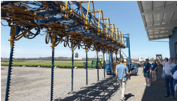
Woodburn Nursery & Azaleas has a one-of-a-kind 60-foot autonomous trimmer that's driven by GPS and tilts its blades to cut foliage in pyramids or cones. It wasn't cost effective for the nursery to trim every block of trees twice by hand, but the trimmer covers that much work easily.
