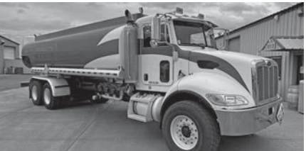
1-2007 PETERBILTS PB 340, CUMMINS ISC, 315 HP, 10 SPD TRANS, 4:63 REAR RATIO, 295 75R 22.5 DRIVE RUBBER, 385 65R 22.5 STEERS 70%, 90% BRAKES, ALL ALUMINUM WHEELS, 2006 4500 GAL PROGRESS ALUMINUM FUEL TANK, MC 406 AL, 3 COMPARTMENTS, 1000, 1500, 2000, 1 DELIVERY SYSTEM WITH LCR II ELECTRONIC METER, BOTTOM LOAD, VAPOR, SCULLY, 2 HOSES, 150” OF 1 1/4 HOSE OR 100’ OF 1 1/2, VALVE TO SWITCH BETWEEN SIZES. STK#4121 .....
