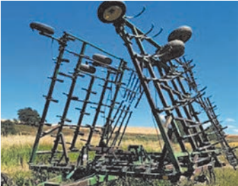
JD 980 Cultivator 41', 6" spacing, single point depth control.....$11,000
