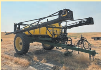
'14 BESTWAY FIELD PRO 4, 100' Booms, 1600 Gal Tank, AutoBoom, Triple Nozzles.....$17,950
