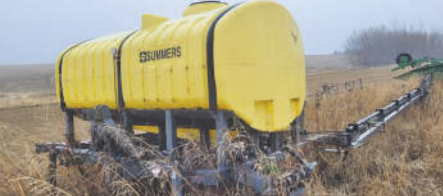
DEMCO RM600 3-POINT SPRAYER, 65', 600 Gal, 5 Section Boom Control, Greentronics Autoboom ..... $18,500
